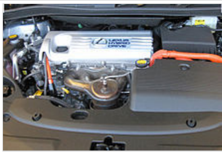
HS 250h inline-four engine with electric motors
